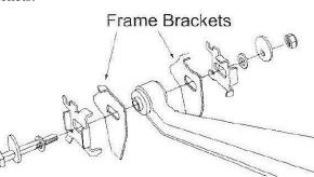
11. Torque nut to 85ft. lbs. Set toe and road test vehicle.
